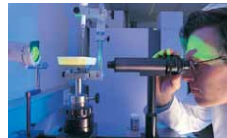
"Dr. Wax" Leif Torgersen Axell (1943-2012) measures contact angles between water and wax.
