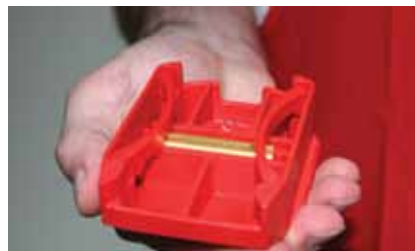
SWIX SUPER RILLER (T0401) with 1 mm blade.
